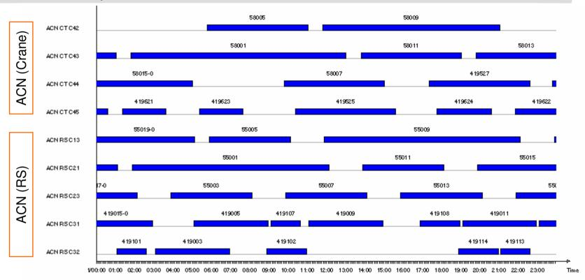
All loading tracks are in use in the timetable simulation. But there are reserve capacities, mainly in tracks C32 and C42, as buffer for the timetable simulation.
