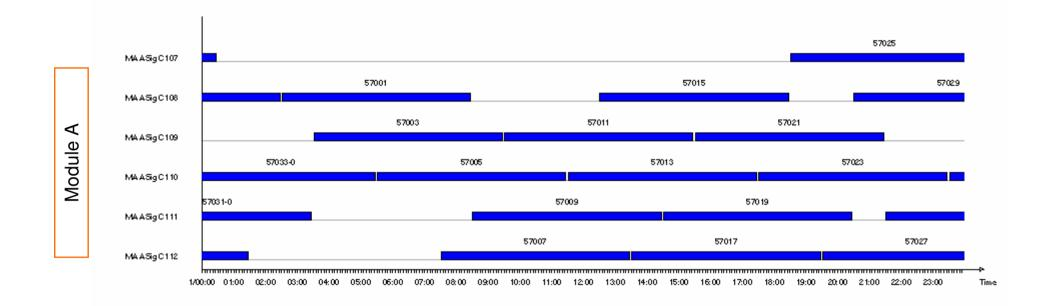
All tracks are in use in timetable simulation. Loading track C107 is occupied only up to 25 % and will serve as buffer in multiple simulation (with delays).
