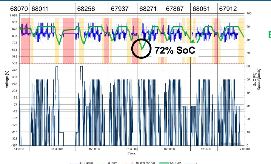
Voltage, Speed, and Battery State of Charge
