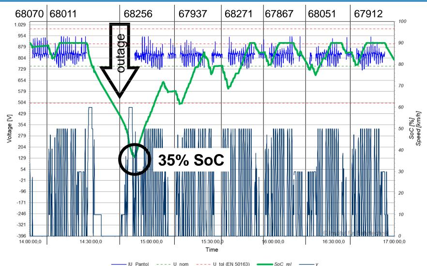
Voltage, Speed, and Battery State of Charge
